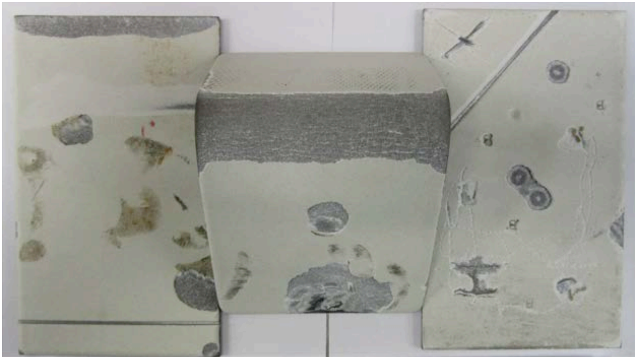
Figure 1 – EonCoat panels with intentional mechanical damage.
