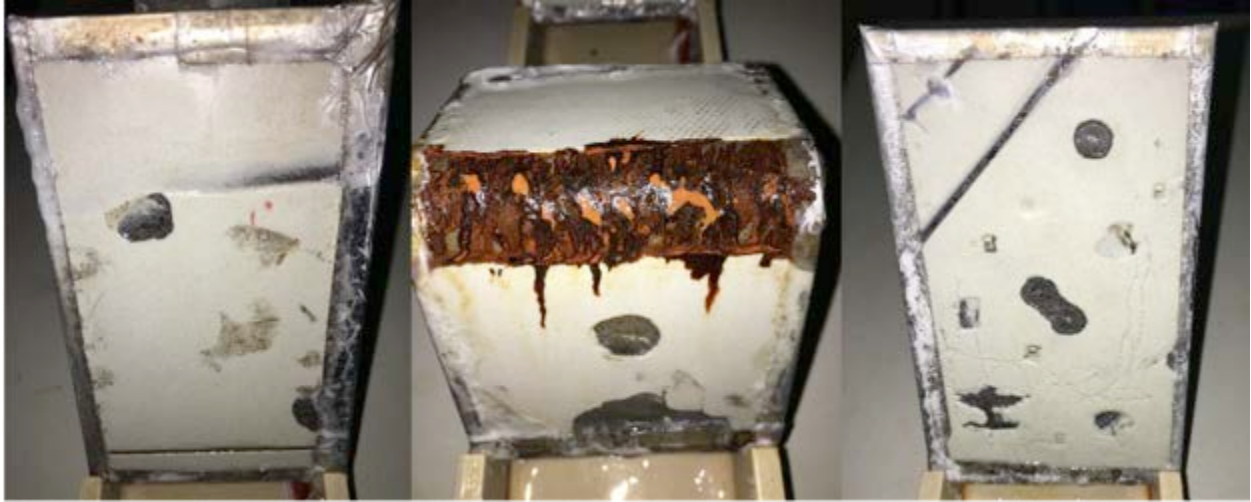
Figure 2 – EonCoat panels with intentional damage after 335 hours of B117 exposure.
